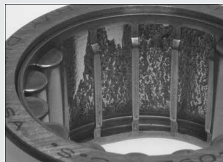
Fig. 38. The housing bore was machined with an improper taper, causing the uneven load distribution and GSC spalling in this cylindrical roller bearing outer ring.
