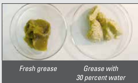
Fig. 74. The effect of water on grease is depicted here.
