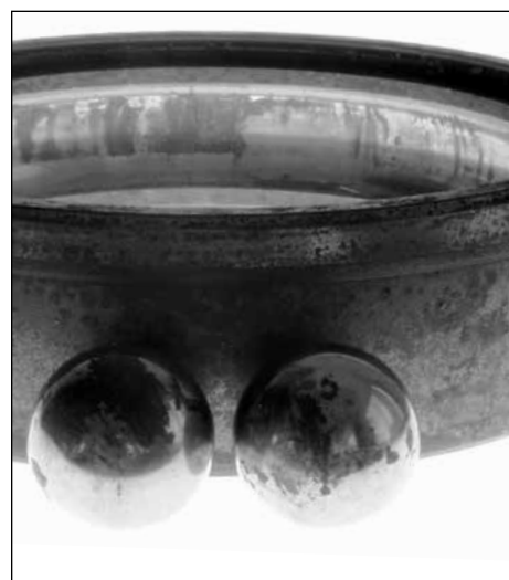
Fig. 16. This ball bearing outer race also depicts etching and corrosion.
